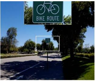
Bioptic mode positions a rectangle at the top center of the screen that allows you to magnify a specific section of the screen without losing the greater context of the view in front of you.
