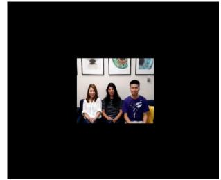
This mode allows you to change the Field of View (FOV) of the screen. This helps individuals with Retinitis Pigmentosa or Glaucoma to be able to see better by shrinking the entire image into a smaller viewing area.
