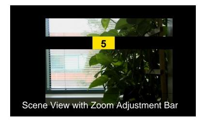
Once an adjustment bar is on the screen (see image above), then you can use buttons 3 and 4 to move the adjustment bar to the left and right. You can then use button 1 to close the adjustment bar and apply the currently selected value. Alternatively, you can wait 10 seconds without pressing any buttons, and the adjustment bar will go away and apply the currently selected value.
