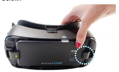
**NOTE:** When the Display Unit is connected correctly to the headset, if voice prompts are enabled (see page 42), it will say "**Device inserted correctly**." If there is no verbal confirmation, the Display Unit is not connected correctly and the headset controls will not respond. Ensure that the device speaks before you close it securely into the headset.
