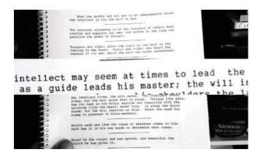
Reading Line mode presents text in black letters on a white background. It also provides a magnification bar in the center of the screen to magnify one or more lines of text while allowing a normal view above and below the bar. Increase the size of the reading line by slowly swiping up on the touchpad. Swipe down on the touchpad to decrease the size of the reading line.
