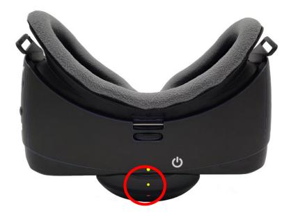
The screen will turn black a few minutes after you set the headset on the charger. When the Display Unit is fully charged, you will hear a verbal prompt, "Charging completed" (if voice prompts are enabled, see page 42). The IrisVision Live's battery lasts, on average, 3 hours. It can last 3+ hours without continuous use, and all day (8 to 10 hours) on standby. You can make the most of this time by powering the headset off when not in use.
