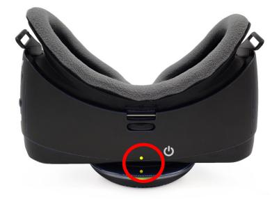
If the IrisVision Live is powered on, you will hear a audible confirmation that the device is charging.
