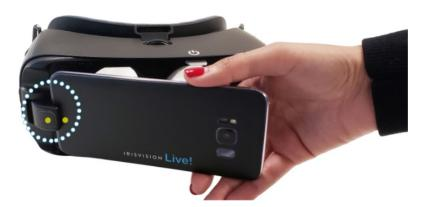
2. Securely lock the Display Unit into the headset by pushing the Display Unit against the spring lock, as shown below.
